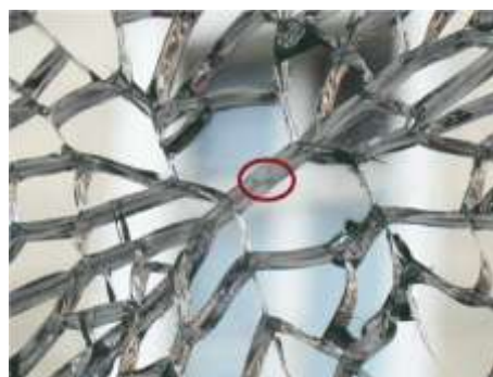
Sample. Spontaneous breakage
