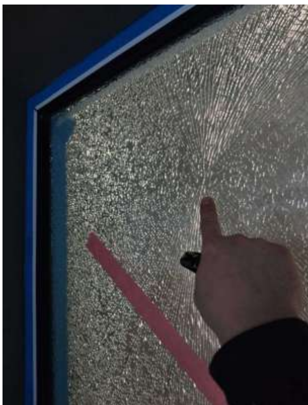
Sample. Spontaneous breakage
